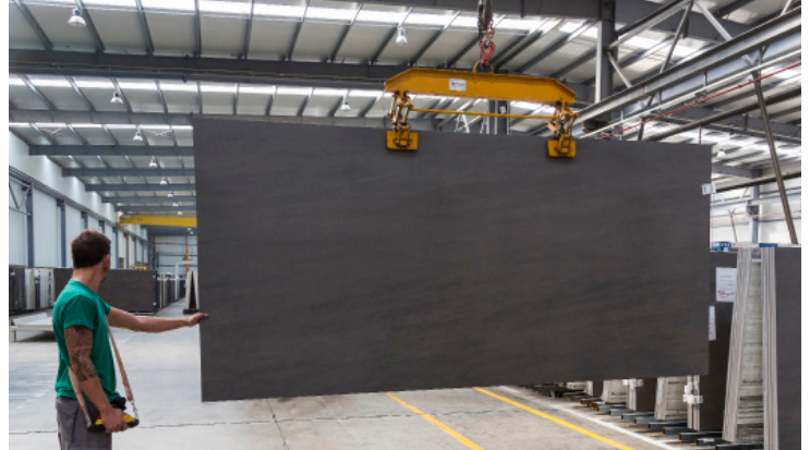
Image 2: Neolith slab handling with Clamp
